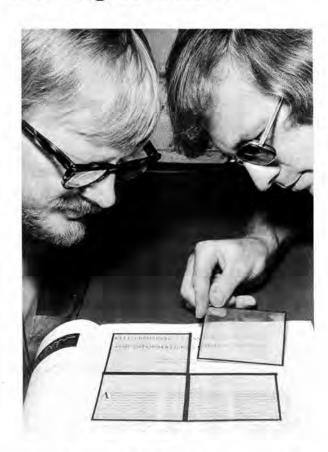
TRANSPARENCY of PLZT material is demonstrated here by Tom Cutchen and Jim Harris (both 2521). The segments will be assembled into an aircraft window together with sensors and circuitry that enable the window to turn opaque so that the aircrew is protected from thermal burn and flashblindness. They were fabricated in Sandia's Ceramics Shop (7122-1) under the direction of Gary Snow (2521) and Bob Dungan (7120).
